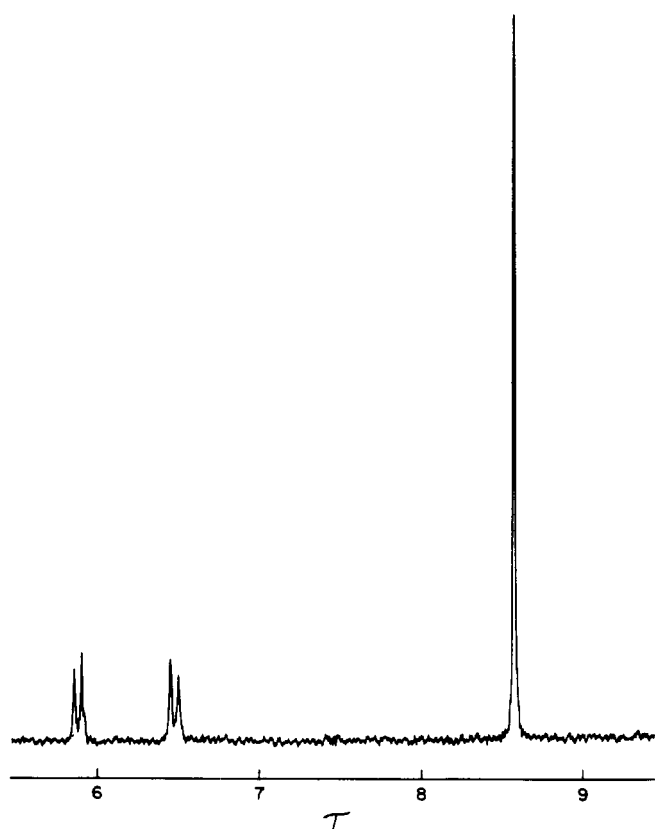
Figure 2. 220 MHz nmr spectrum of dicryl metabolite M-1 (aliphatic part); solvent: chloroform.
